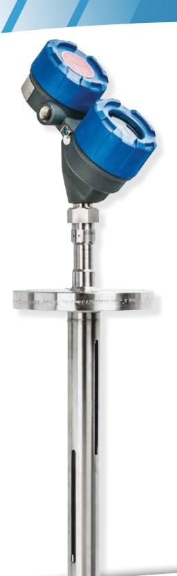
Guided Wave Radar is based upon the principle of Time Domain Reflectometry (TDR). TDR utilises pulses of electromagnetic energy, which are transmitted down a probe. When a pulse reaches a liquid surface that has a higher dielectric than the air/vapour in which it is traveling, the pulse is reflected.
