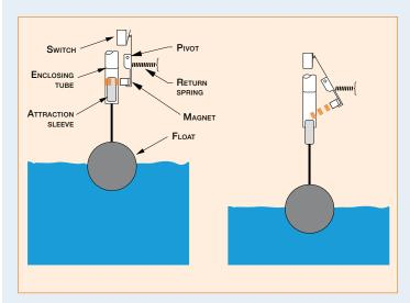
T20 - T21 Liquid float level switch
