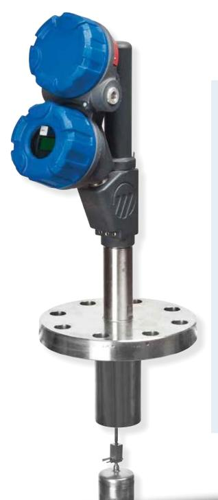
The buoyancy force works on the displacer which will vertically move in (increasing liquid level) and out (decreasing liquid level) the linear differential transformer (LVDT). Due to this movement voltages are induced in the secondary windings of the LVDT. These signals are then processed in the electronic circuitry and used to control the output signal.
