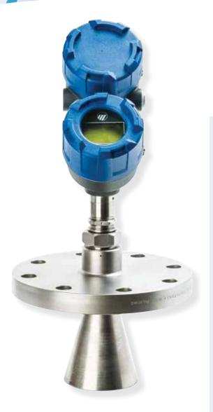
Pulse Burst Radar emits short bursts of energy to a liquid surface. Ultra-high-speed timing circuitry measures the time of the signal reflected off the liquid surface.
