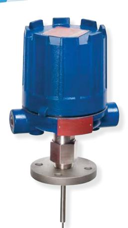
A permanent magnet is attached to a pivoted switch actuator. As the float/displacer rises following the liquid level, it raises the attraction sleeve into the field of the magnet, which then snaps against the non-magnetic enclosing tube, actuating the switch. The enclosing tube provides a static pressure boundary between the switch mechanism and the process. On a falling level, the float/displacer deactivates the switch.
