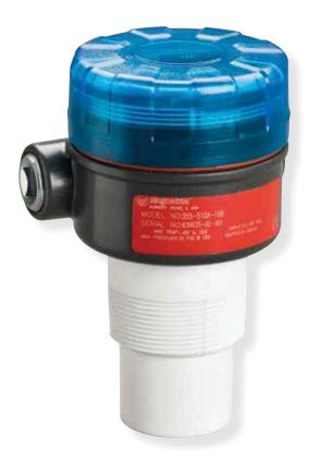
The level measurement is accomplished by emitting an ultrasonic pulse from the transducer face and measuring the elapsed time between sending this pulse and its reflected echo from the liquid surface. Since the speed of sound is temperature dependant, the transducer also measures ambient temperature to compensate for the changing velocity.
